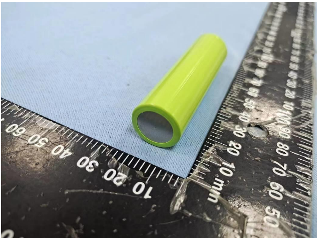
Picture 10 Bottom view of cell (Model: INR18650L26)
