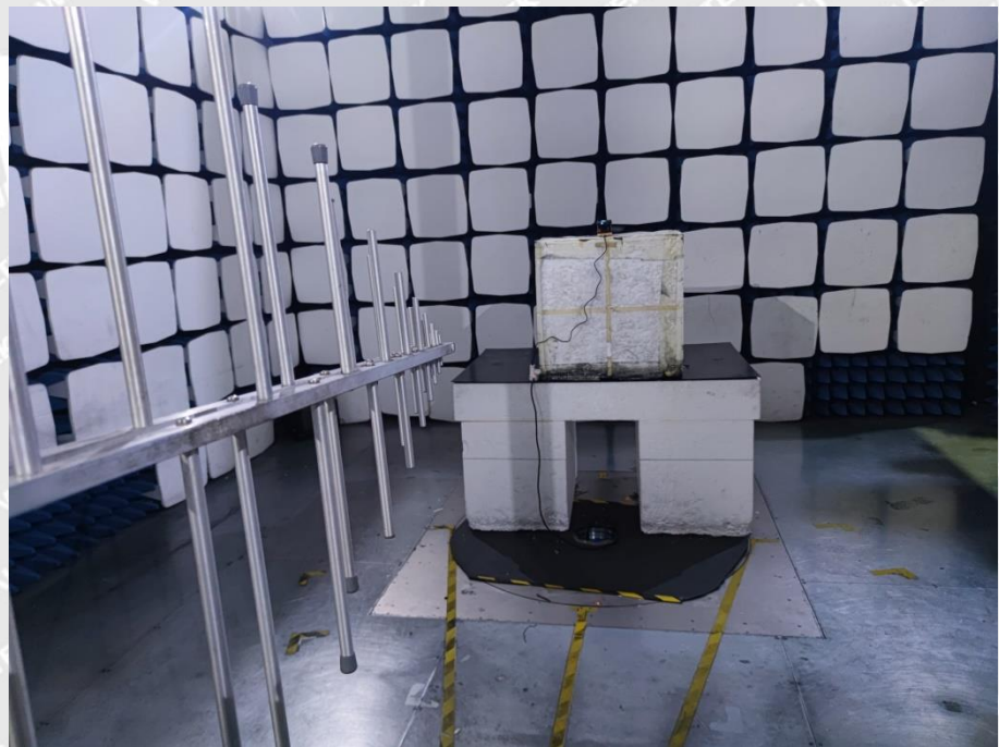
Radiated Spurious Emission Test Setup (Above 30MHz)
