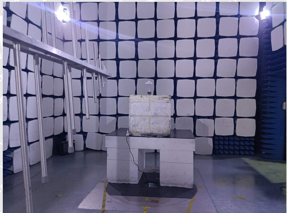
Radiated Spurious Emission Test Setup (Above 30MHz)
