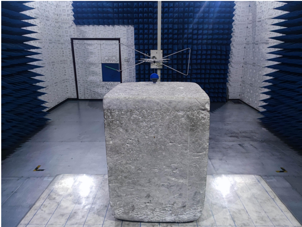
RADIATED SPURIOUS EMISSION TEST SETUP
