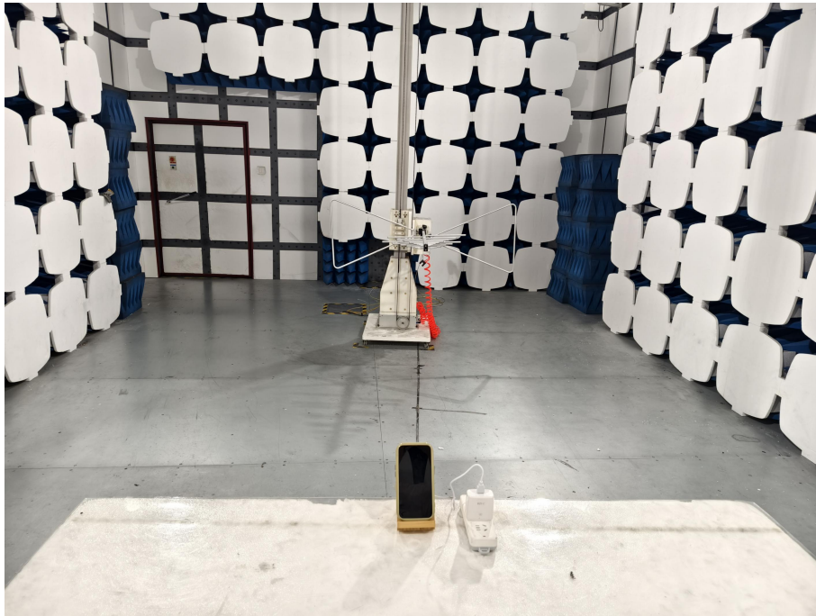
Photo of Radiated Emissions Measurement
